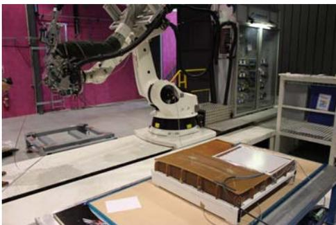
*Compositadour 16 fibre laser automated Fibre placement cell*
